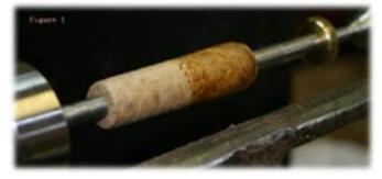
Figure 2: Collecting sanding dust with 180 grit to use for the CA slurry as a sealer. This step could be omitted and a sanding sealer used. The slurry works exceptionally well for open grain woods.
