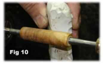
Figure 11: Buffing the white diamond with a clean, soft, dry cloth. This is a rag from a box of rags purchased at the paint store…it is cotton T-shirt material.
