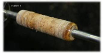
Figure 5: Remove the excess slurry with around nose scraper, and then sand. Use your regular sanding routine.
