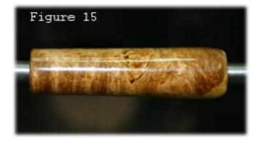
Figure 12: Application of HUT Ultra Gloss Plastic Polish...Apply on lathe and buff with a clean, soft, dry cloth. Any plastic polish could be used as well a scratch and swirl remover automobile polish.
