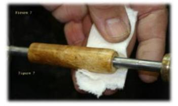
Figure 7: Applying the CA from the bottle. The opaper towel oil applicator is underneath the blank and the CA bottle is on top. Move from one side to the other applying a bead of CA...One pass only is enough CA.
