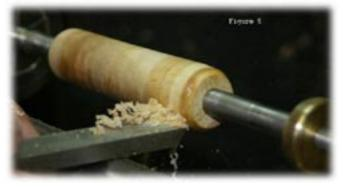
Figure 6: Applying the boiled linseed oil...3 drops...too much oil can lead to failure...A common cause of failure, blotches, ghosting, and globing. The amount of oil may need to be adjusted for your shop conditions. Three drops is not an absolute, but works for me.
